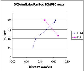
The figure at the right illustrates the difference in energy use, as a function of watts/cfm, between a PSC and ECM motor on a typical fan powered terminal.
